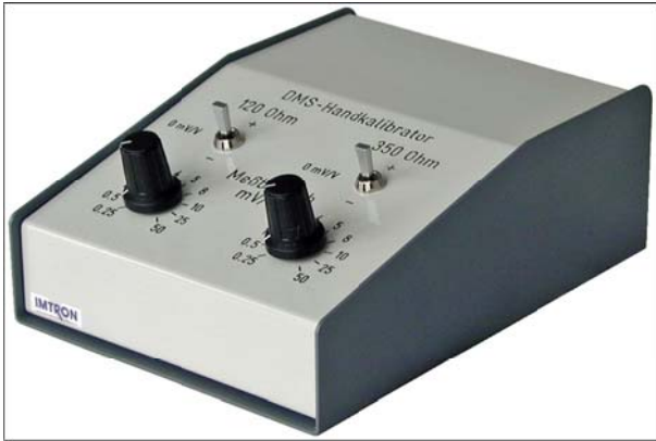
Picture with 2 bridge resistances
